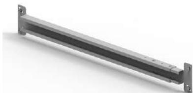
Telescopic connecting piece for SF/SK /SL/ SM/TL/TM and TT lifting columns. The traverse can be easily pushed into the grooves (width 8 mm) of the lifting column and clamped with a hexagonal wrench.
