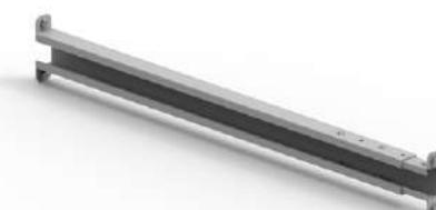
Telescopic connecting piece for SK /SL/ SM/TL/TM and TT lifting columns. The traverse can be easily pushed into the grooves (width 8 mm) of the lifting column and clamped with a hexagonal wrench.
