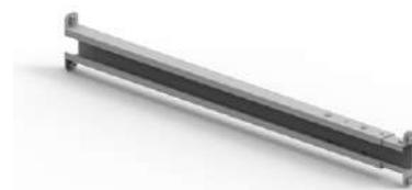
Telescopic connecting piece for SK /SL/ SM/TL/TM and TT lifting columns. The traverse can be easily pushed into the grooves (width 8 mm) of the lifting column and clamped with a hexagonal wrench.
