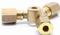
To connect two pressure elements with one cylinder the Y-connection is needed. The lifting speed will be doubled but the lifting load will be halved.
